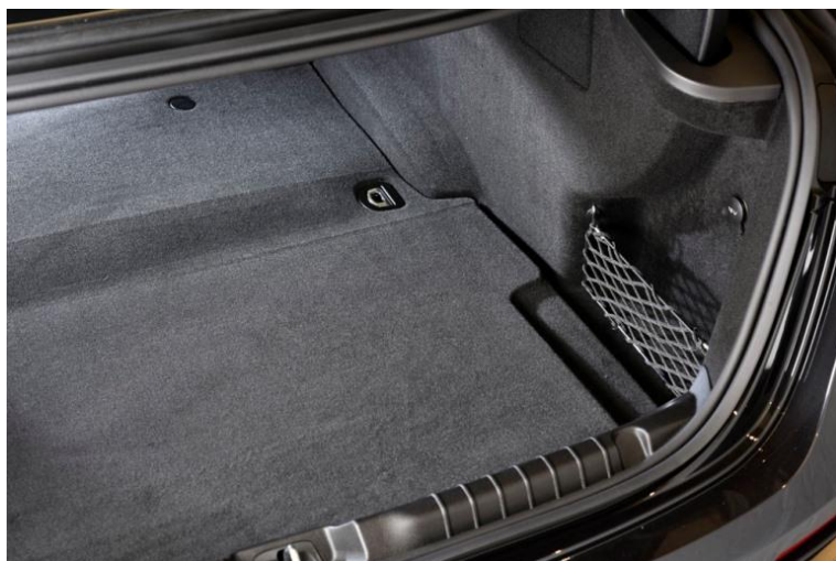
Load floor made with RENOLIT GORCELL . (Photo: RENOLIT COMPOSITES , PR002)
